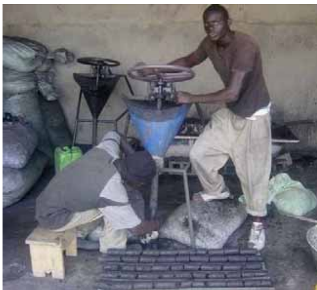
Briquetting residues using the rotor press (Photo: PERACOD)
