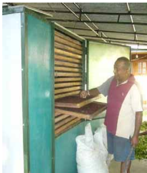
Spice drying racks (Photo: Practical Action)
