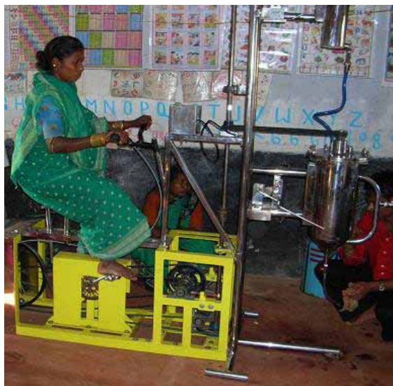
Pedal-driven biodiesel reactor (Photo: CTxGreEn)
