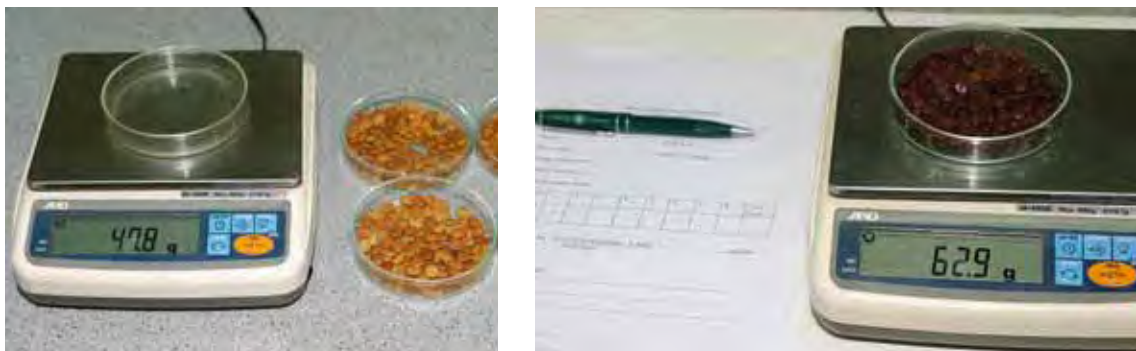
Figure 12.7 Seed weight determination test samples
