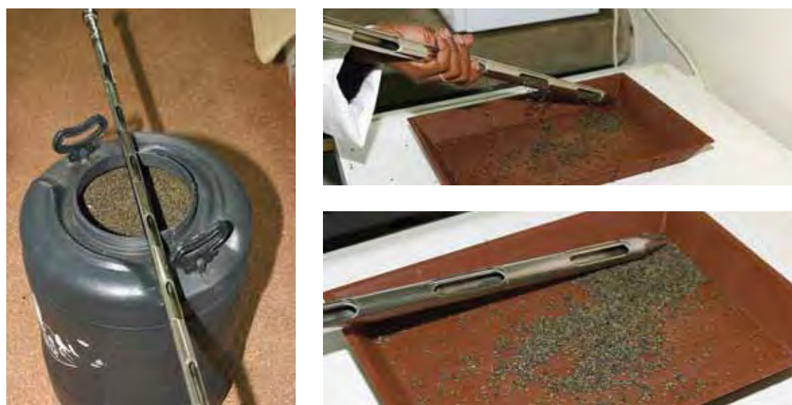
Figure 12.1 Seed sampling for purity analysis using a sleeve type trier
