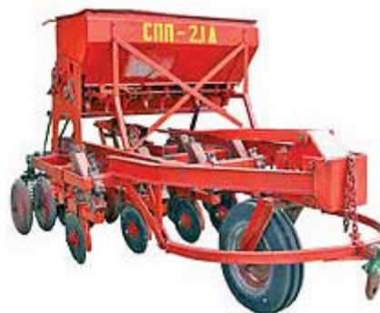
No-tillage direct drill equipment (left: planting legumes on wheat stubble, leaving most of the straw on the soil surface; right: locally made equipment from northern Kazakhstan).
