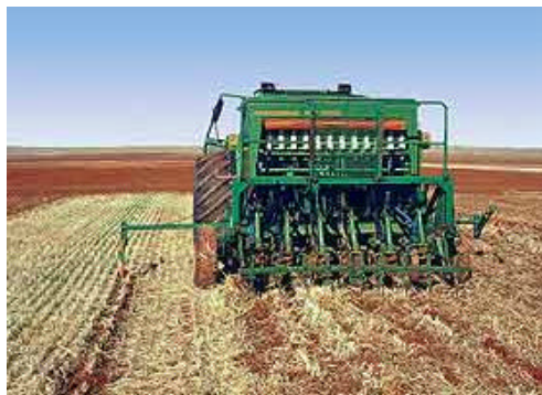
No-tillage direct drill equipment (left: planting legumes on wheat stubble, leaving most of the straw on the soil surface; right: locally made equipment from northern Kazakhstan).
