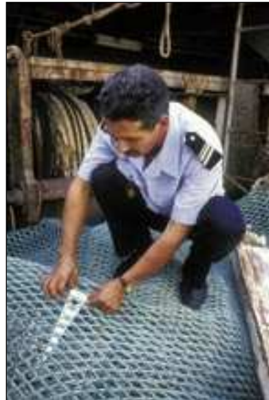
An inspector at Agadir port, Morocco using a gauge to measure stretch mesh in the codend of a trawl net.
