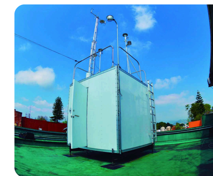
Automatic station for air quality monitoring. Julio C. Martínez Hernández
